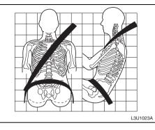
The lap part of the belt should be worn low and snug on the hips, just touching the thighs. In a crash, this applies force to the strong pelvic bones so you'd be less likely to slide under the lap belt. If you slid under it, the belt would apply force at your abdomen. This could cause serious or even fatal injuries. The shoulder belt should go over the shoulder and across the chest. These parts of the body are best able to take belt restraining forces.
